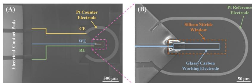
Scanning electron micrograph of an E-Chip<sup>2</sup>
