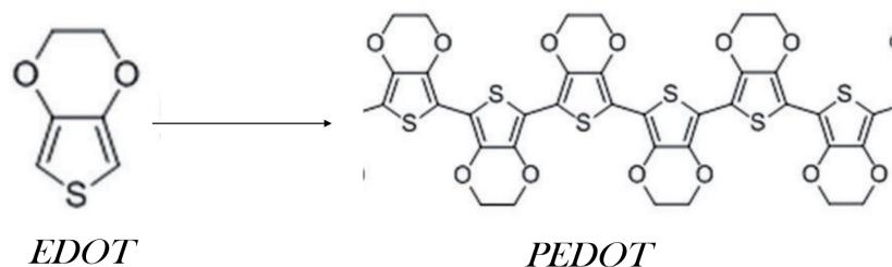
Polymerization reaction of PEDOT
