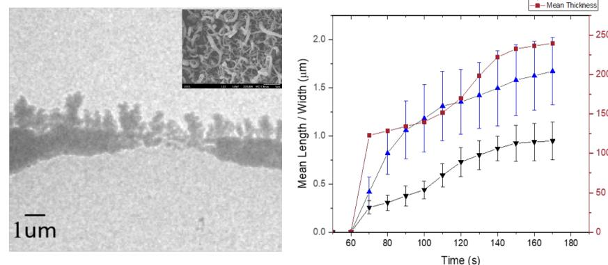
Nucleation and growth of PEDOT with a fibrillar morphology using in-situ TEM (inset: SEM of PEDOT:PAA nanofibrils)
